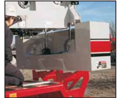
Fast & efficient hydraulic counterweight removal enhances roadability
