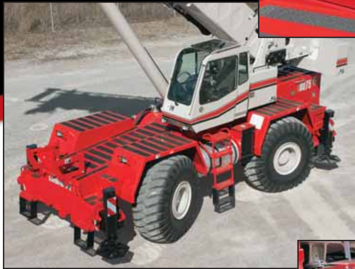
Fast & efficient hydraulic counterweight removal enhances roadability
