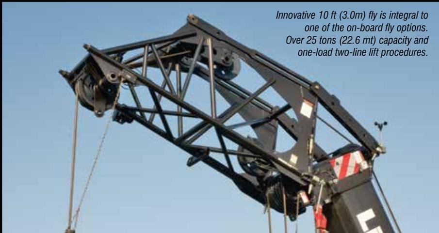
*Innovative 10 ft (3.0m) fly is integral to one of the on-board fly options. Over 25 tons (22.6 mt) capacity and one-load two-line lift procedures.*
