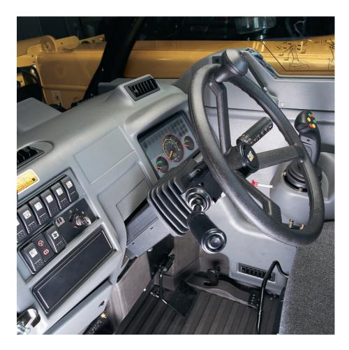
**Enclosed Cab.** The TH210 is equipped with an enclosed cab allowing the operator to work comfortably, with air conditioning available as an option. The cab structure has been designed and certified to provide falling object and rollover protection (FOPS/ROPS).
