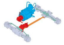
**Hydrostatic Drive.** The TH210 features a high pressure, closed circuit hydrostatic drive to deliver powerful but smooth acceleration while providing continuous torque through the two speed ranges. The low speed band is 8 km/h (5 mph) and the high speed band is 32 km/h (20 mph).
