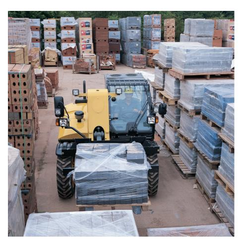
Steering Modes. Three steering modes (circle, two wheel and crab steer) allow the operator to easily position the machine in small, confined areas. Steering modes are selected by using the steering mode switch in the operator's compartment. An indicator light in the cab illuminates when the wheels are properly aligned.
