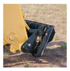
**Manual Coupler.** The TH210 utilizes a manual quick coupler using the same interface as the Caterpillar Skid Steer Loader.
