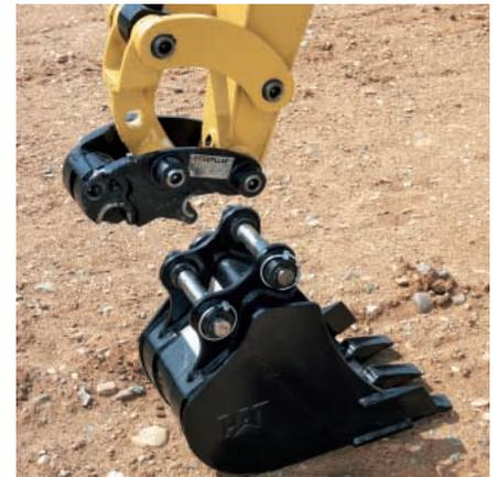
**Mechanical Quick Coupler.** The Cat Quick Coupler makes frequent tool changes fast and easy. Compatible with all Cat Mini Hydraulic Work Tools, it features a strong, lightweight, low profile design with no debris traps for years of secure work tool changes.
