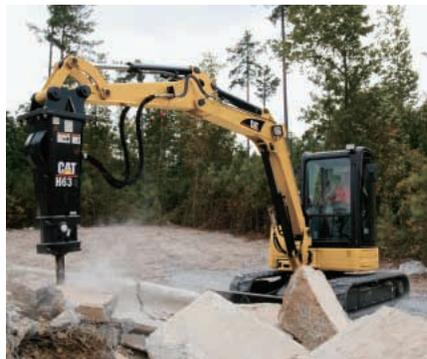
**Auxiliary Lines and Connectors.** The auxiliary lines and connectors including quick connections are fitted as standard, meaning the Cat 303.5C CR come ready to work. Hammer (one-way) and auger (two-way) auxiliary lines are also fitted as standard.
