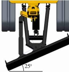
**Versatility and Productivity.** The Cat C Series machine can be made even more productive by ordering the angle dozer blade configuration.
