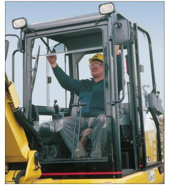
Excellent visibility to the work tool and machine surroundings is provided by the large glass area. The operator's all-round field of view is maximized by the superior cab design and the low hood to the rear.
