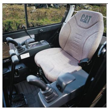
**Low effort pilot hydraulics** and ergonomically designed controls minimize fatigue and maximize comfort for the operator. There is a control pattern changer available as an option. The automatic swing lock helps ensure that the superstructure is held in a secure position while transporting the machine.
