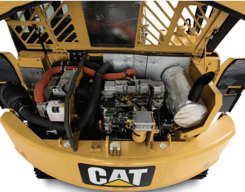
Robust, reliable and easily serviceable are the key attributes of Cat® Mini Hydraulic Excavators. Full steel body work panels and protected front linkage lines are routed neatly out of the way of potential damage above the boom. Easy access to all daily service points are accessed through the rear hood and side cover. A 500 hour engine oil change period lowers operating costs and the Cat S•O•S<sup>SM</sup> points assist easy oil sampling for preventative maintenance checks.
