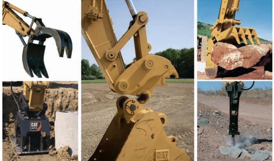
**Hammers.** Cat hammers deliver very high blow rates, increasing the productivity of your tool carriers in demolition and construction applications. Wide oil flow acceptance ranges make Caterpillar hammers suitable for a wide range of carriers and provide a system solution from one safe source.
