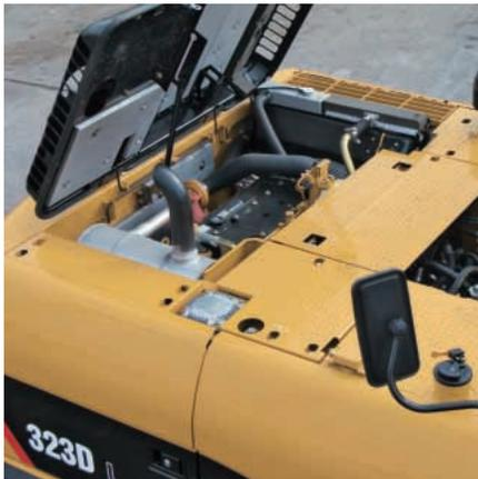
**Performance.** The Cat C6.4 with ACERT™ Technology offers more engine power, and runs at lower speeds for better fuel efficiency and reduced wear.
