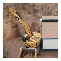
**Heavy Duty Buckets.** Heavy-duty (HD) buckets are used for a wide range of moderately abrasive applications such as mixed dirt, clay and rock. HD buckets have best loading and dumping characteristics and will empty easier in cohesive material. More robust construction than the GP buckets.
