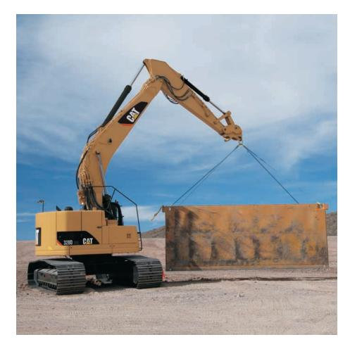
**Auxiliary Hydraulic Valve.** The auxiliary valve is standard on the 328D LCR. Control Circuits are available as attachments, allowing for operation of high and medium pressure tools. These include shears, grapples, hammers, pulverizers, multi-processors and vibratory plate compactors.
