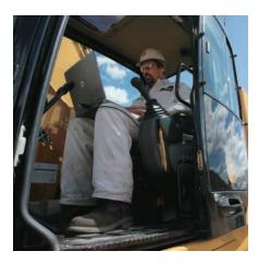
**Diagnostics and Monitoring.** The 328D LCR is equipped with  $S \cdot O \cdot S^{SM}$  sampling and hydraulic test ports for the hydraulic system, engine oil, and for coolant. A test connection for the Cat Electronic Technician (Cat ET) service tool is located in the cab.
