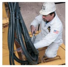
**Greasing Points.** A concentrated remote greasing block on the boom delivers grease to hard-to-reach locations on the front.
