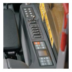
**Console.** Redesigned consoles feature a simple, functional design to reduce operator fatigue, ease of switch operation and excellent visibility. Both consoles have attached armrests with height adjustments.
