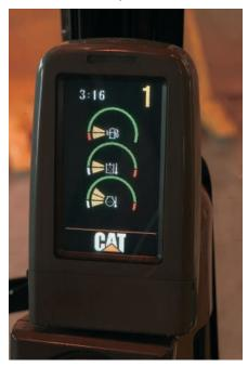
**Monitor.** The monitor is a full color 400x234 pixels Liquid Crystal Display (LCD) graphic display. The monitor angle is adjustable to minimize sun glare and is capable of displaying information in twenty-seven different languages.
