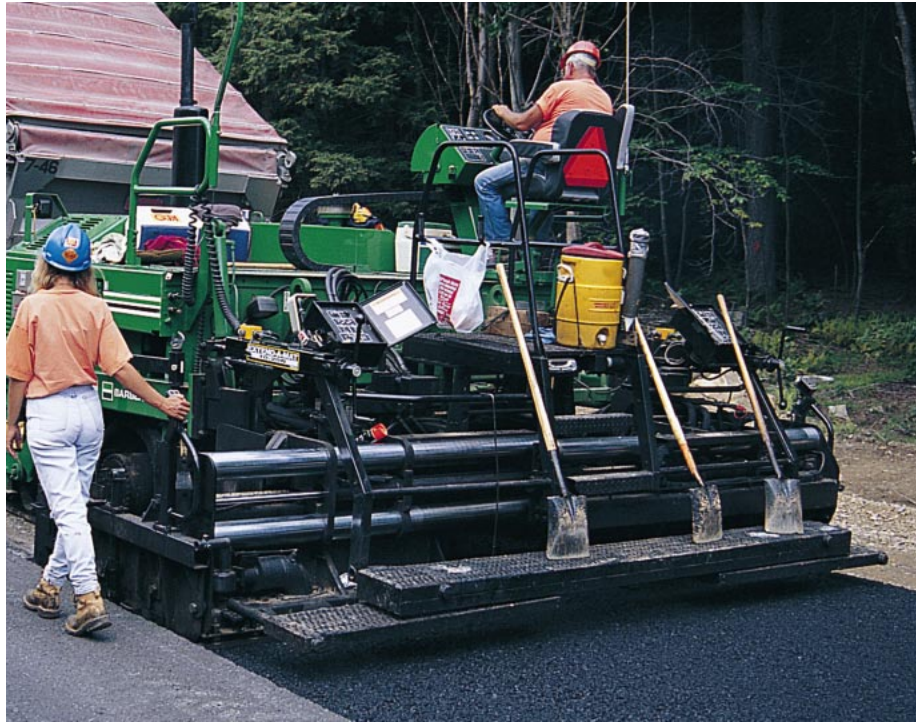
Extend-A-Mat Screed shown with BG-2455C Asphalt Paver.
