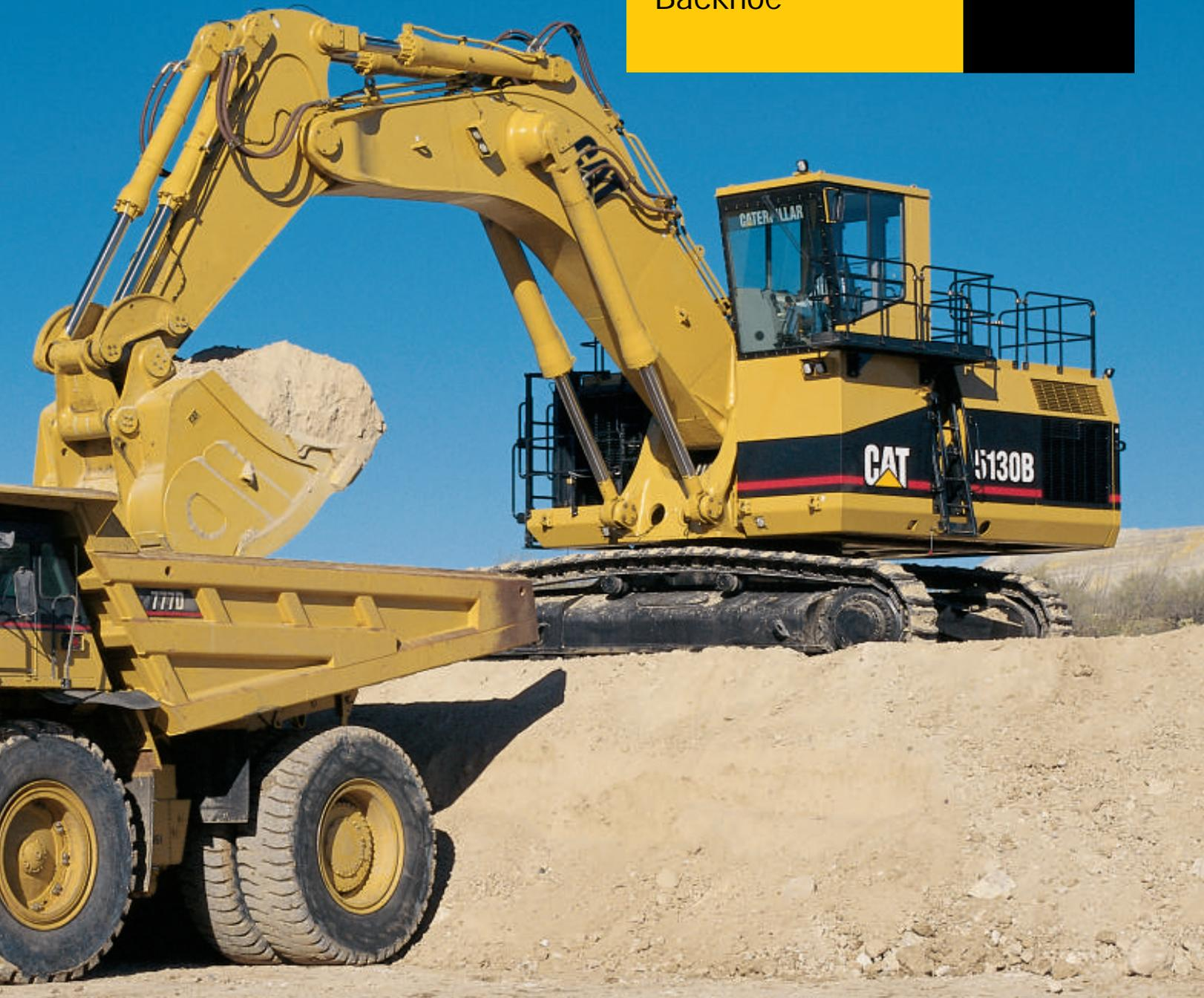
Available in Front Shovel and Backhoe configuration, the new Caterpillar® 5130B is primarily matched to the Cat® 777D truck, but can also be teamed with the 773D or 775D and other trucks in the 65 to 100 ton size class. This makes for efficient loading and hauling systems for mining, quarrying and heavy construction applications.
