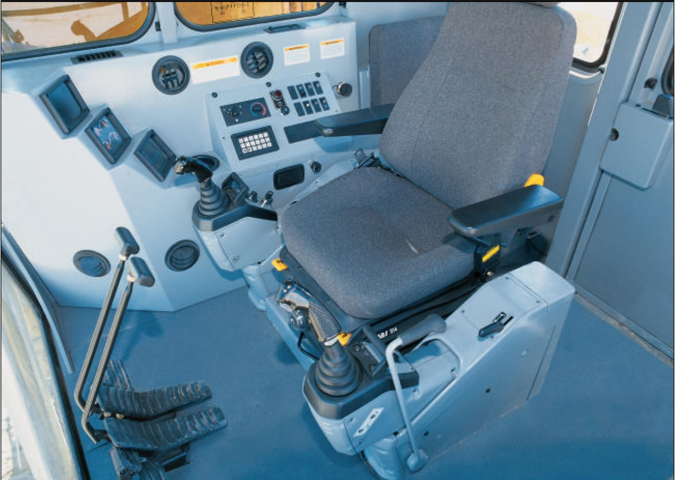
Spacious operator compartment measures 1790 mm (5'10") wide by 2178 mm (7'2") long by 2236 mm (7'4") high and has an exceptional, unobstructed view of the bucket and loading area.
