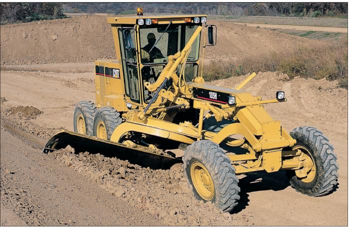
Blade positioning. The blade linkage design provides extensive moldboard positioning. This extended range is most beneficial in mid-range bank sloping and in ditch cutting and cleaning.
