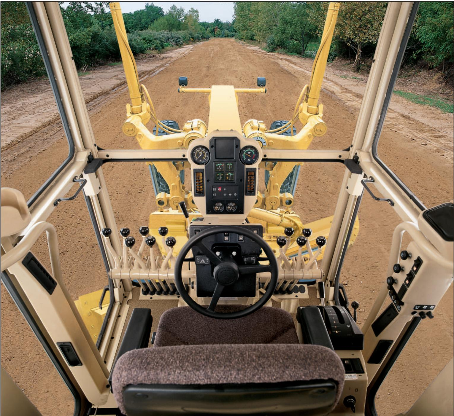
**Exceptional visibility** helps improve operator confidence and productivity. The drawbar has been modified to improve the view through the circle, allowing the operator to see the material as it rolls along the moldboard without leaning. Large side windows allow a clear view of the moldboard heel and tandem tires. A wide rear window and tapered engine hood provide a good view to the rear of the machine.
