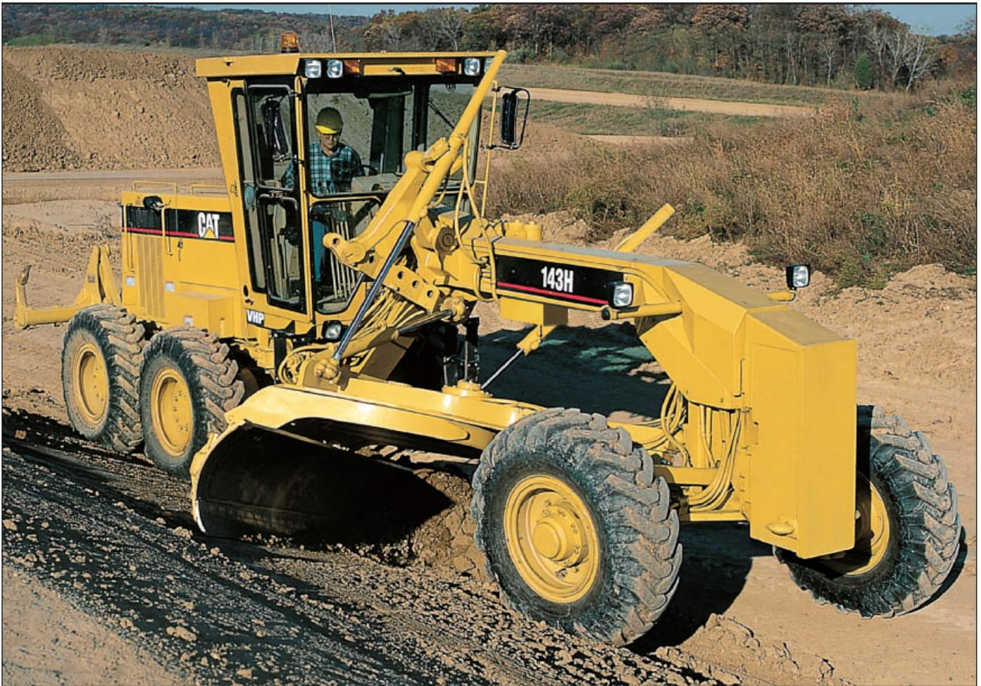
**Blade positioning.** The blade linkage design provides extensive moldboard positioning. This extended range is most beneficial in mid-range bank sloping and in ditch cutting and cleaning.
