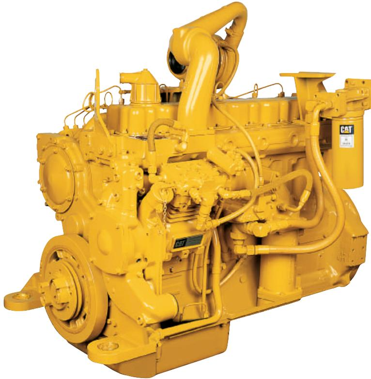
**Cat 3306 engine** continues its tradition of powerful, efficient performance and unmatched reliability and durability. The six-cylinder engine is turbocharged with a high displacement-to-power ratio. This large displacement produces better lugging capability, lower internal stresses and extended component life.
