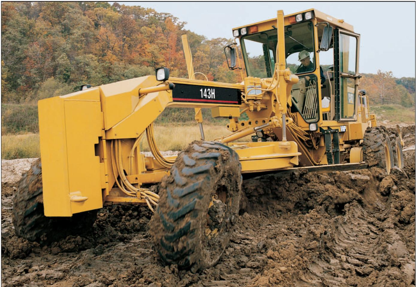
**Superior traction.** All-wheel drive improves tractive performance in poor underfoot conditions such as snow, mud and sand. This feature also provides excellent steering and sidedraft control.
