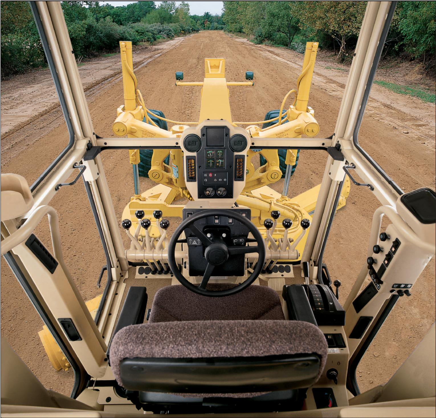
**Exceptional visibility** helps improve operator confidence and productivity in all grader applications. The large front glass area provides an unobstructed view of the moldboard and front tires. The large side windows offer a clear view of the moldboard heel and tandem tires. A wide rear window and tapered engine hood provide good visibility to the rear of the machine, especially to a rear ripper.
