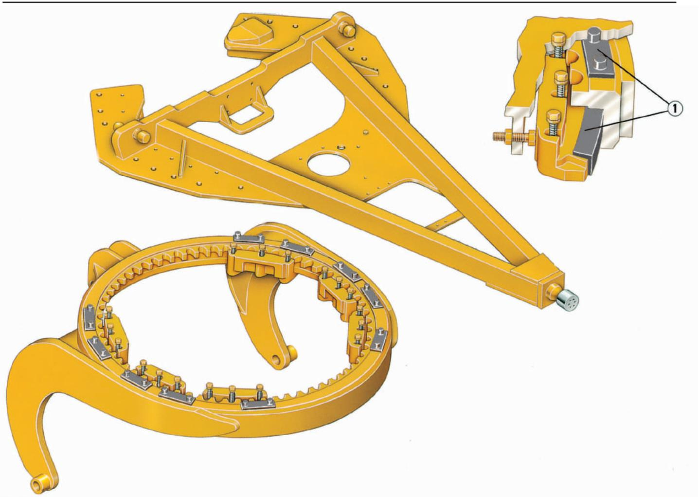
**Rugged construction.** The drawbar features an A-frame, box-section design for high strength. The bottom is machined to provide accurate adjustment and precise blading. A one-piece forged circle is built to stand up to high stress loads. To resist wear, teeth are induction-hardened in the critical areas. For maximum support, the circle is secured to the drawbar by six support shoes.
