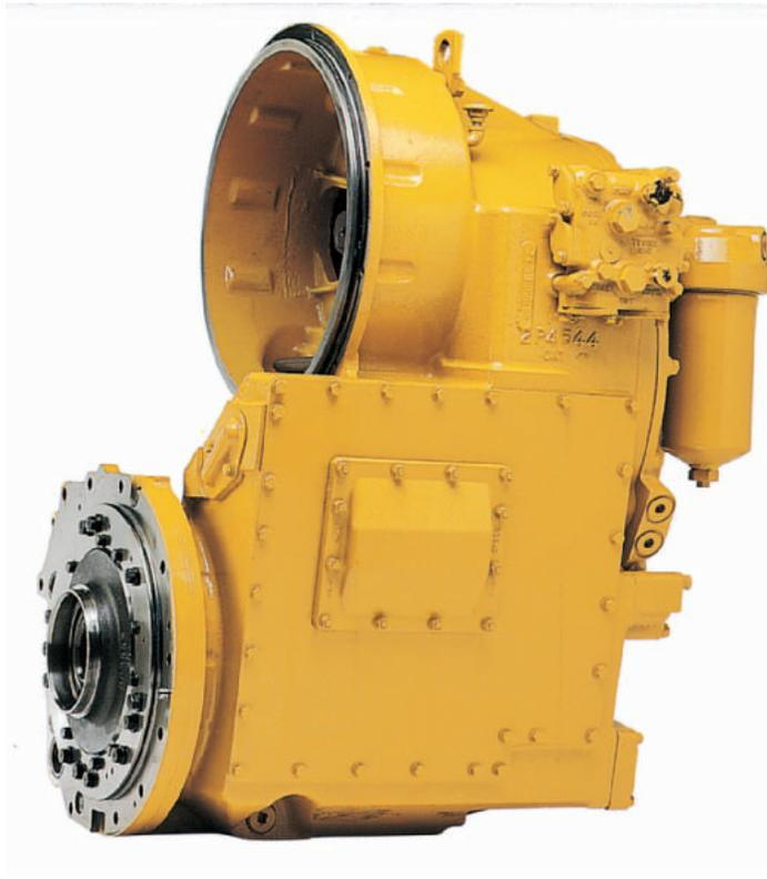
**Power shift transmission.** Caterpillar designs and builds transmissions specifically for Cat motor graders. The transmission provides on-the-go, full-power shifting as well as inching capability.
