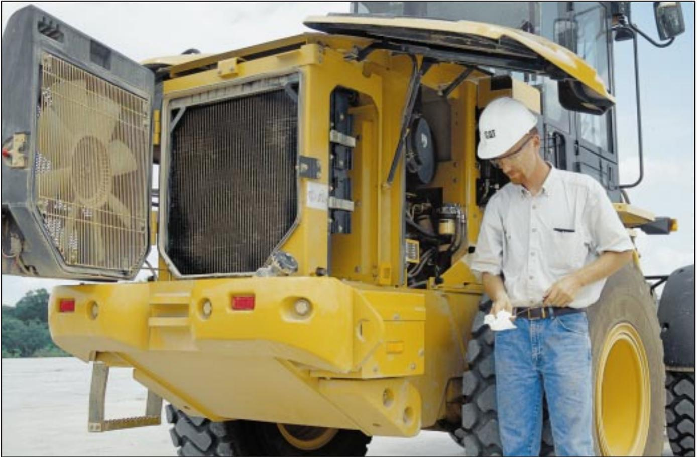
**Easy, wide open access.** Gull-wing doors with pneumatically-assisted lift cylinders effortlessly lift up for exceptional access to major power train components. All filters and service points are within easy reach.
