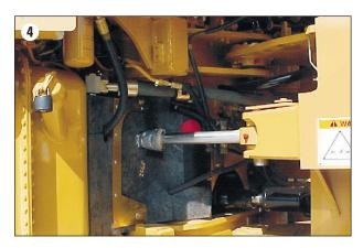
**Tilt Cylinder Guard** protects the tilt cylinder from material that may damage the cylinder during refuse handling applications.
