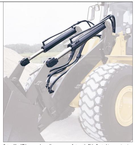
Caterpillar XT hoses and couplings are uniquely designed and tested to work together as a system for superior performance. Hoses are specifically engineered and manufactured for high abrasion resistance, excellent flexibility and easy installation. Caterpillar couplings use O-ring face seals which provide positive sealing for reliable leak-free connections. Reliable components reduce the risk of leaks and blown lines, helping protect the environment.
