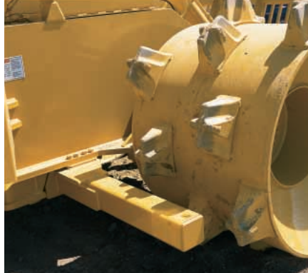
Striker Bars. Are located in front of and behind the rear wheels and behind the front wheels. They provide substantially improved protection from trash that can be thrown or carried by the wheels.
