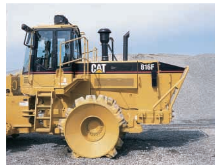
Left Side Platform. Provides easier access to the rear of cab.
