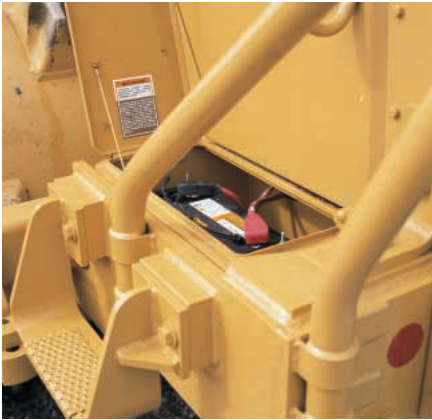
Integral Rear Bumper. Helps protect radiator, fan, batteries and engine.
