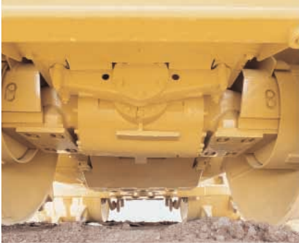
Hinged Engine and Power Train Guards. Help prevent trash build-up and shield components from demolition debris, trash, wire, rebar and harmful chemicals.
