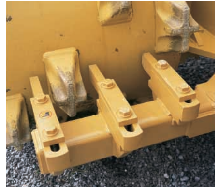
Optional Wheel and Tip Cleaner Fingers. Are welded onto the standard striker bars. These fingers keep the wheels from plugging when working in cohesive materials such as clay or mud.
