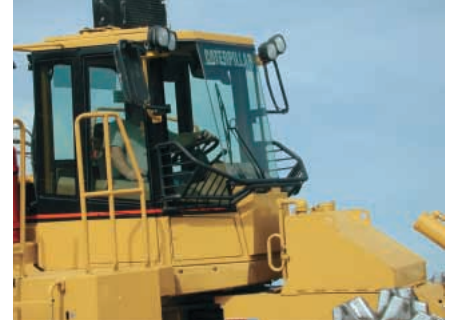
Optional Front Window Guard. Across the bottom of the front cab glass prevents debris from damaging the lower portion of the front windows.
