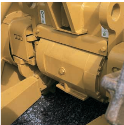
Standard Axle Guards. Prevent trash build-up on axles and protect axle seals.
