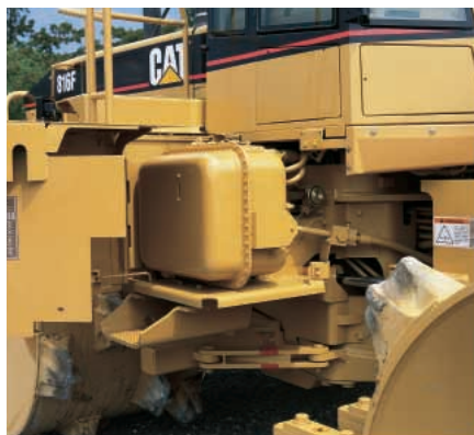
Hydraulic Tank and Steering Cylinders. Are guarded to resist damage.
