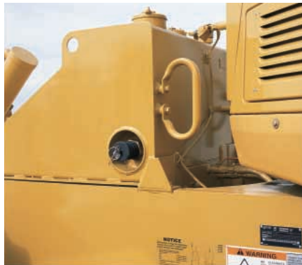
Fuel Tank. Is positioned away from debris and easily reached.
