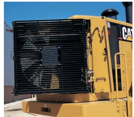
**The Reversing Demand Fan** is a speed controlled, hydraulic fan that provides maximum cooling efficiency. Power is directed through the fan system only when it is needed and reverses automatically to purge debris. (Pressing rocker switch in cab may also manually reverse fan.)
