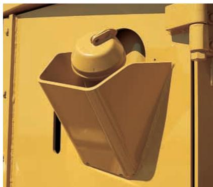
**Hydraulic tank** is guarded to resist damage. Oil sight gauge is visible for easy checking.
