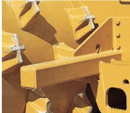
**Striker bars** are in front and behind the rear wheels, and behind the front wheels. They provide substantially improved protection from trash that can be thrown or carried by the wheels. The front also provides for access to the fuel tank in front frame.
