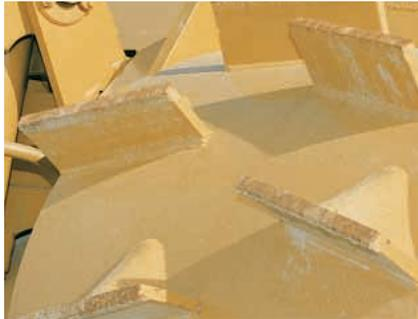
**Self-cleaning Chopper Wheels (optional)** are designed to deliver maximum compaction and traction in landfill work.
