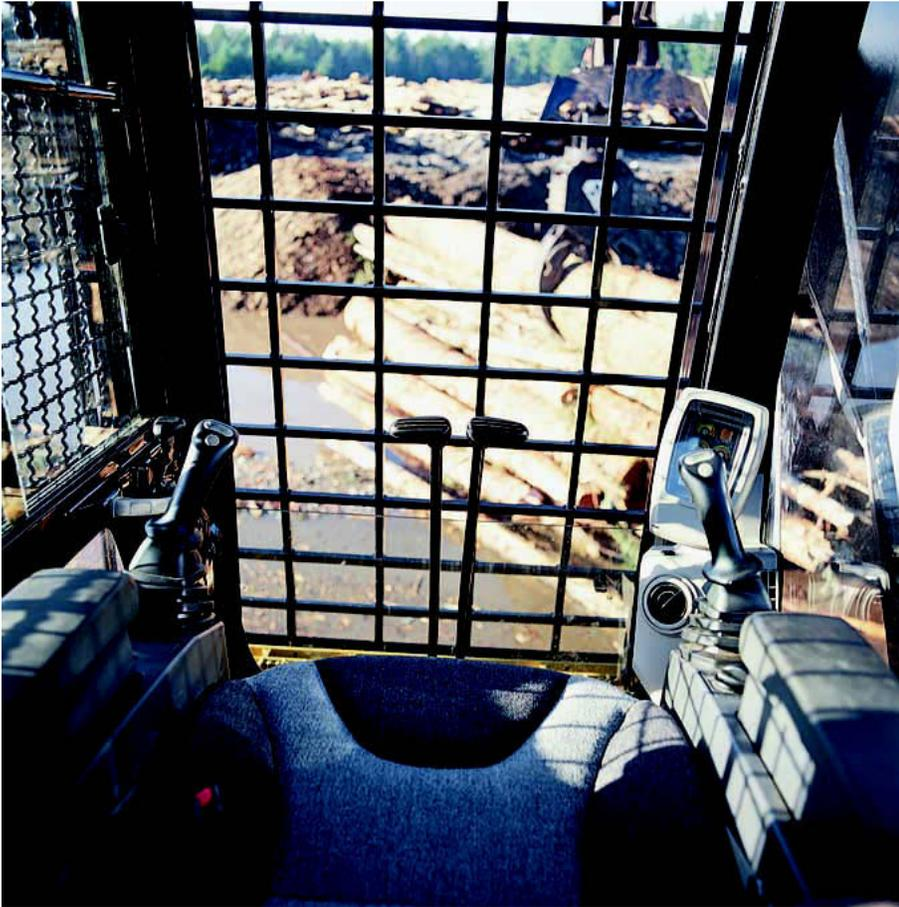
**Operator Station.** The 322C FM operator work station is quiet with ergonomic control placement and convenient adjustments, low lever and pedal effort, ergonomic seat design and highly efficient ventilation.
