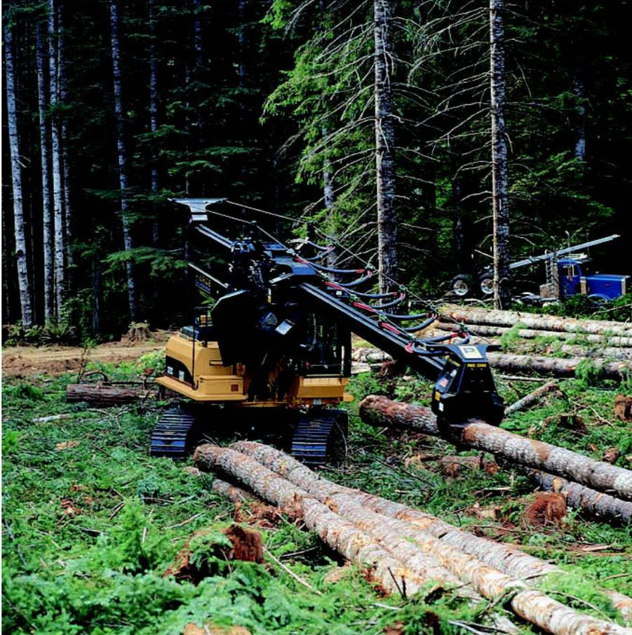
**The Caterpillar Heel-Type Loader Arrangements.** The Caterpillar® heel-type loader arrangements fit a wide variety of log handling and loading applications in the woods and mill yards. Heel booms are especially well-suited for use with large diameter saw logs.
