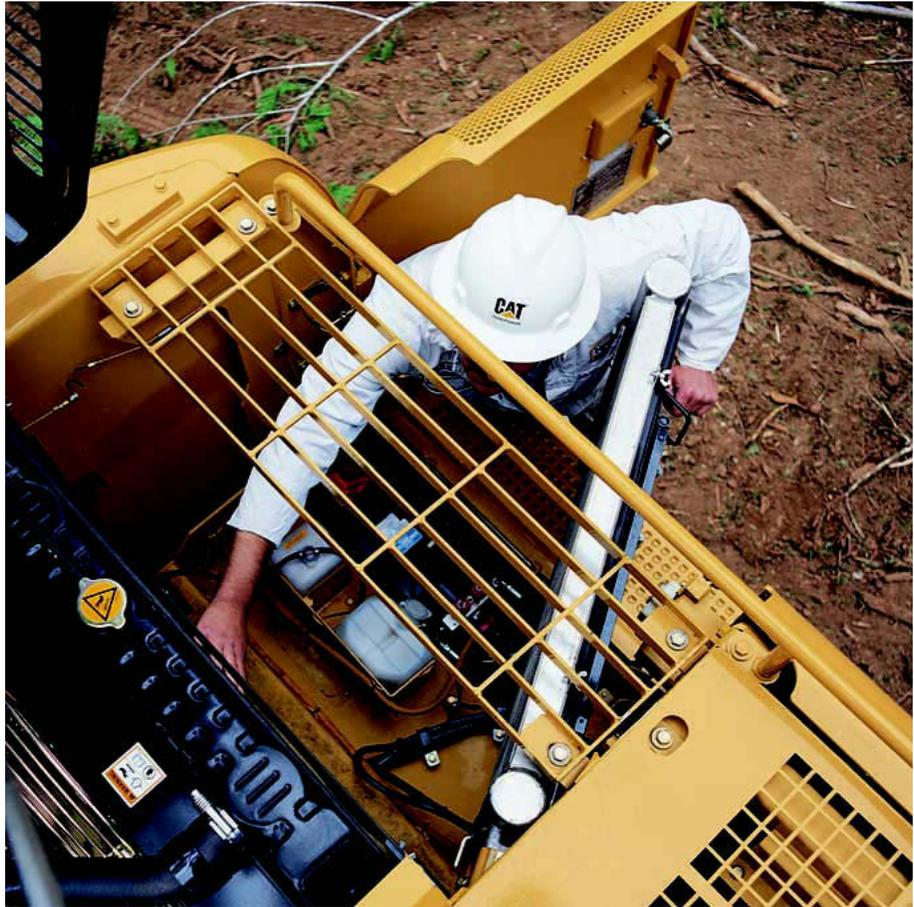
**Diagnostics and Monitoring.** The 322C FM is equipped with S•O•S<sup>SM</sup> sampling ports and hydraulic test ports for the hydraulic system, engine oil and for coolant. A test connection for the Electronic Technician (ET) is located behind the cab.
