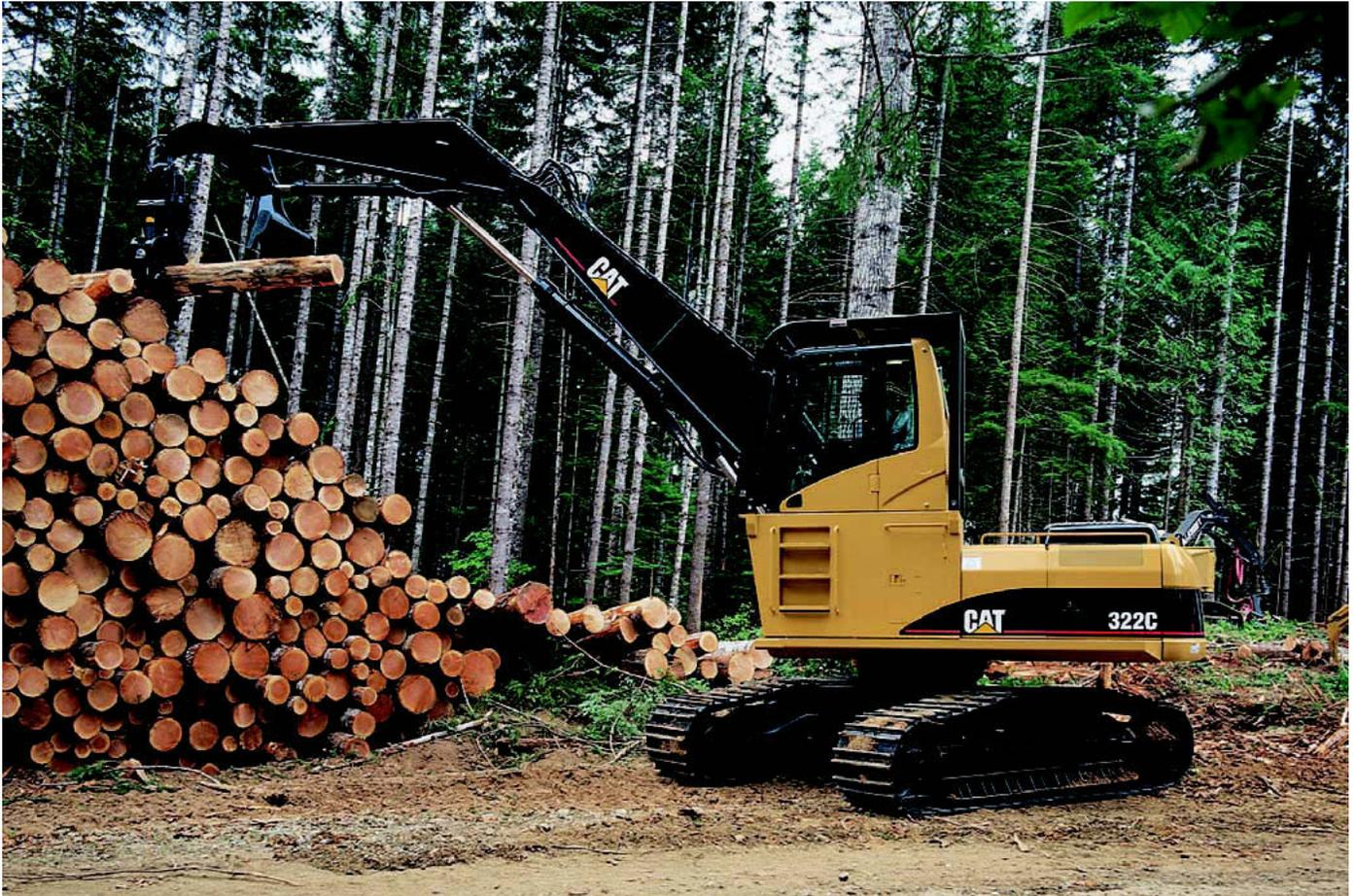
**Heel-Boom Grapples.** Factory-installed and supported heel-boom grapples are matched to the factory logging fronts to increase production and reliability.
