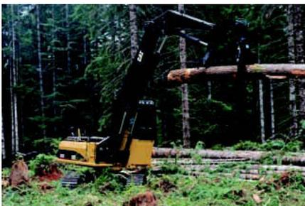
**The Caterpillar Log Loader Is Purpose Built.** The Caterpillar log loader is purpose built for forest applications. Completely assembled, heel-type log loaders (including grapple) are available from the factory.
