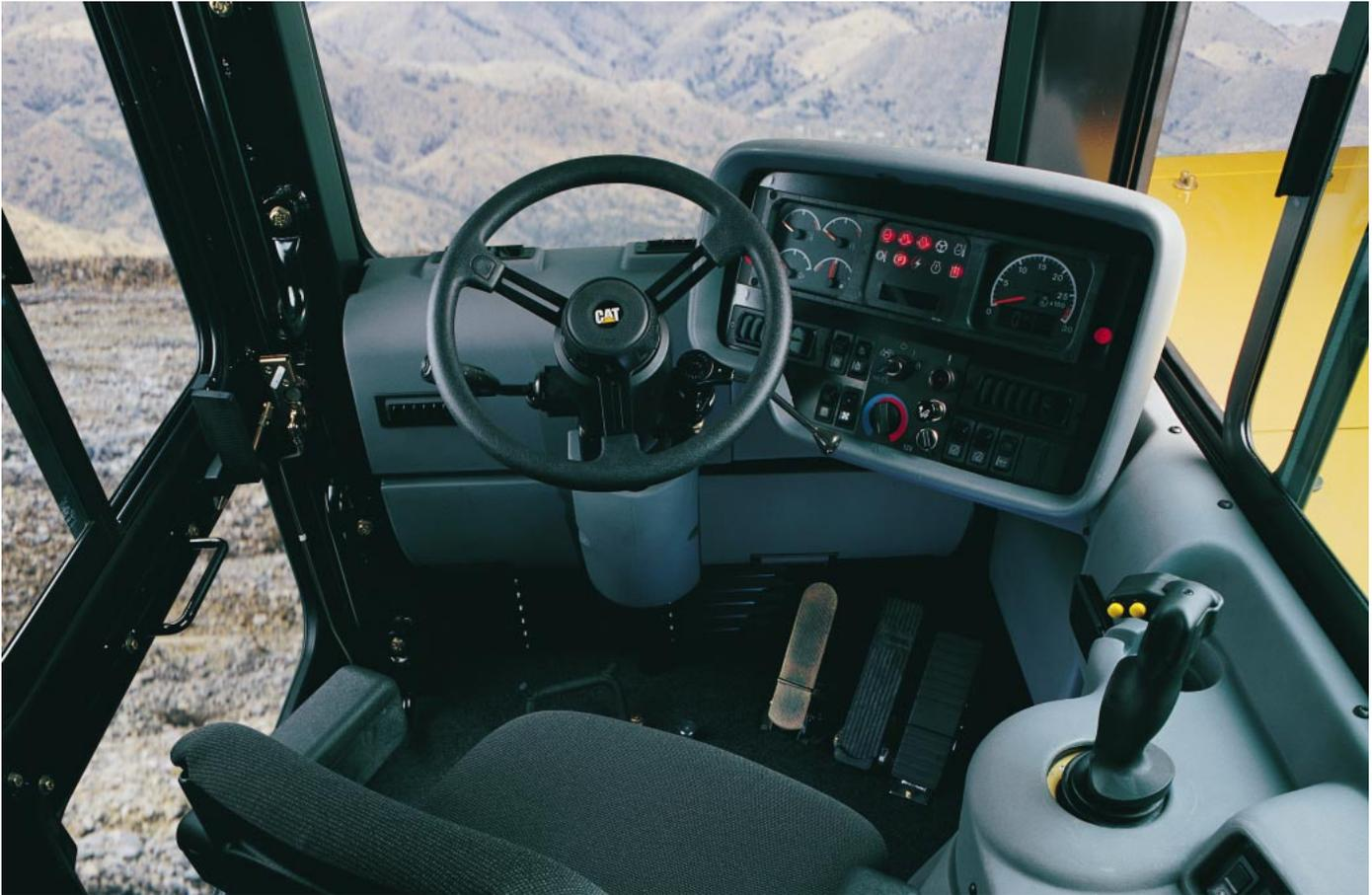
**Sound Suppression.** Sound suppressed, rubber mounted ROPS cab reduces sound and vibration for comfort.
