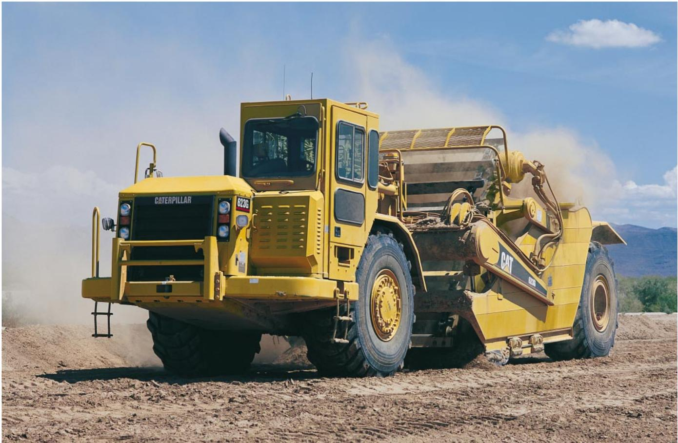
**Material Application.** Work alone capability makes it ideal for picking up windrows, soil mixing, as well as cleanup and production work. Conditions material which promotes compaction in the fill.
