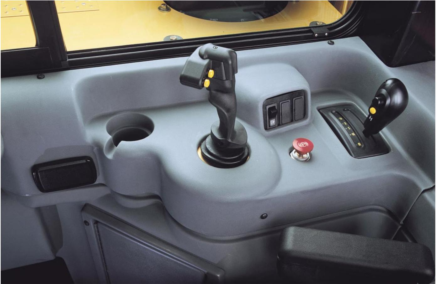
**Joystick Control.** Simple and easy to operate, enhancing the productivity of operators of all skill levels. Requires 25 percent less force to control the critical scraper functions and requires 40 percent less stick movement than before.
