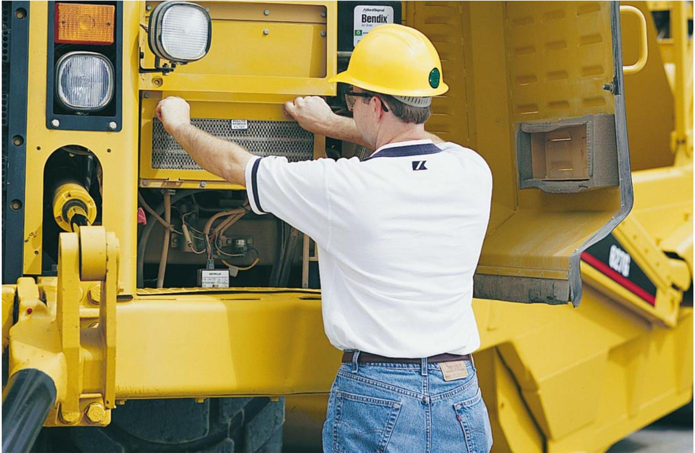
**Service Points.** Service points for the engine are grouped on the right-hand side for easy access.
