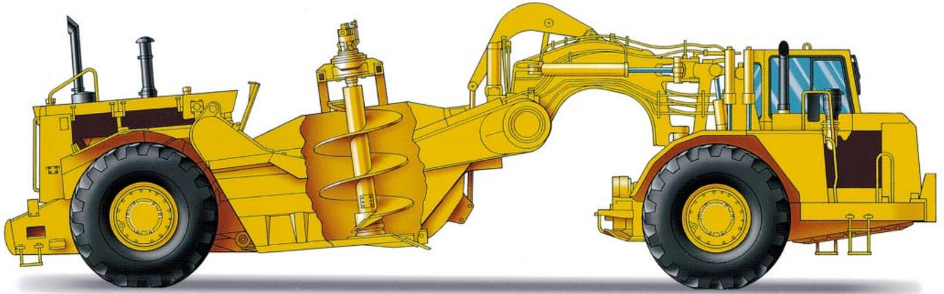
**Material Application.** Work alone capability with a wide material appetite ranging from overburden to laminated rock. Conditions material which promotes compaction in the fill and significantly reduces dust during loading.
