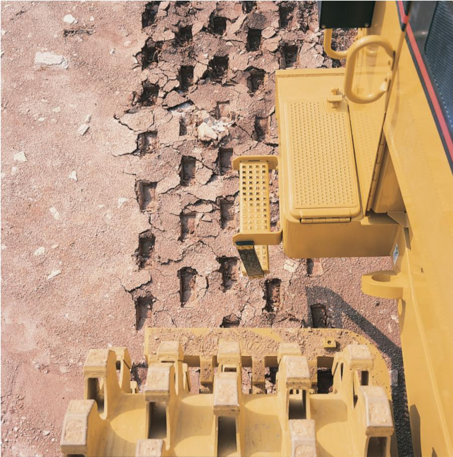
**Wheel Design.** Gives the operator four-wheel width coverage in just two passes with front and rear wheel tracking that eliminates gaps and overlaps.
