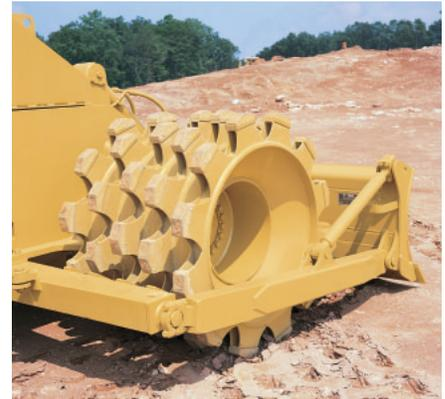
**Outside Mounted S-Blade.** With multiple box section construction including heat treated moldboard and DH-2 steel cutting edges and end bits for long life. The outside mounting is a stronger design because stresses are put on the frame rather than the blade so blade flexing is reduced. It also allows for higher lift and a wider blade can be used than with an inside mounted design.
