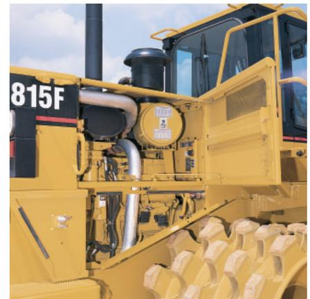
**Right Side Service Access.** Features that are easily reached under the hood include fuel filter and water separator, fuel primer and engine oil dipstick.
