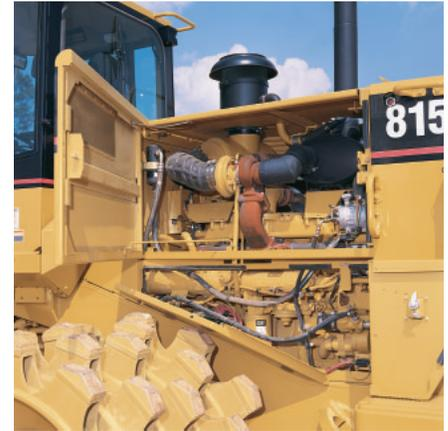
**Left Side Service Access.** Provides convenient entry to the engine oil filter, grease points (lower), air filter (front), power train oil dipstick (top), coolant sight gauge (top), power train oil fill (below cab), power train oil filter and high speed engine oil fill.
