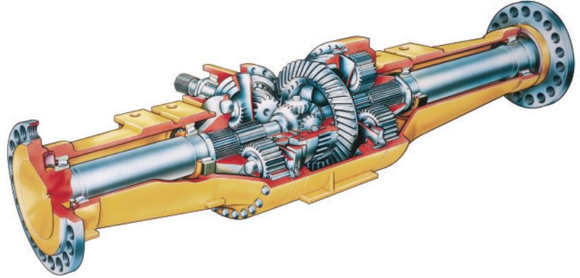
**Front Axle.** Is rigidly mounted to the frame to support the weight of the compactor, internal torque loads and external loads applied during compacting and dozing operations.
