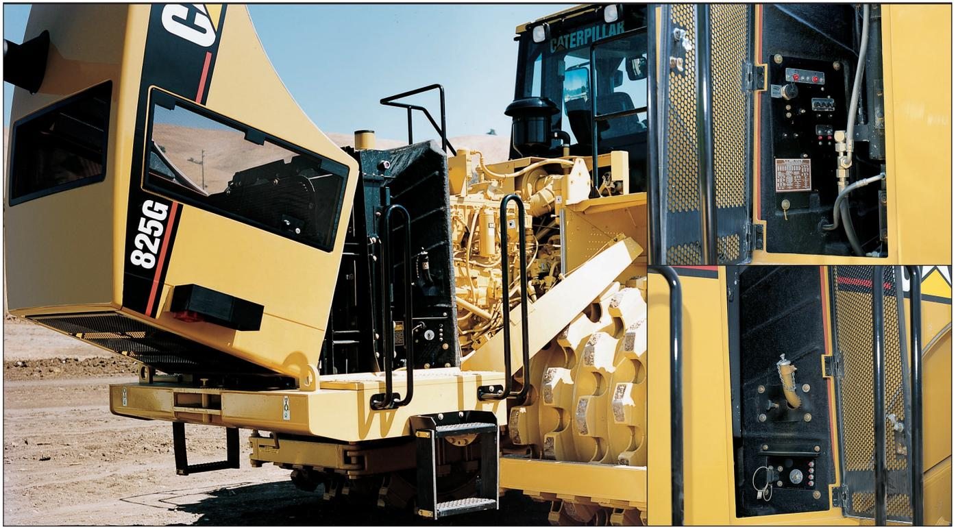
**Daily maintenance** has never been more accessible than on the 825G. Lockable, ground level service doors give quick access to engine oil fill and dipstick, coolant sight gauge, grease fittings for the rear frame, relay panel and electrical breakers. All four maintenance-free batteries are secure in a built-in battery box in the right rear frame. U-joints are lifetime lubricated, leaving the slip joint as the only driveline component needing grease.
