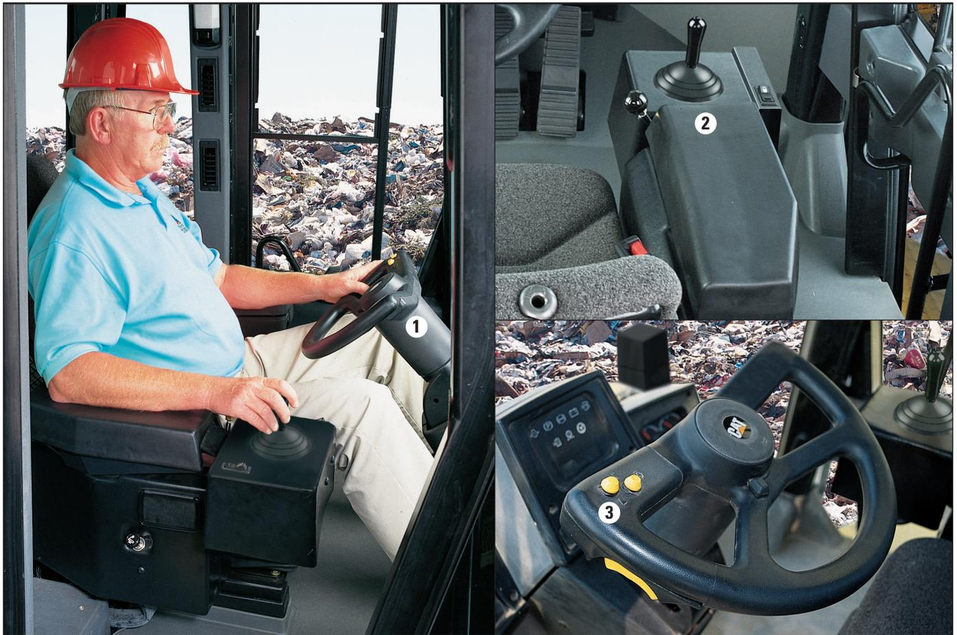
One of the most exciting benefits of the 825G is the dramatic reduction in operator motion effort provided by Command Control steering, integrated transmission controls, low-effort implement controls and fully hydraulic brakes. These features combine to produce the easiest operating machine in its class.
