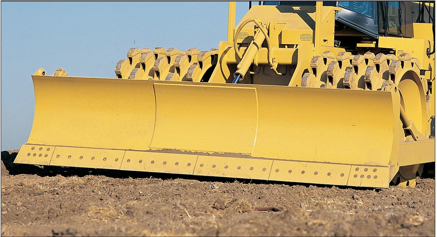
**Does light production** dozing and spreads fill, backfills, stockpiles, charges hoppers, and cleans up around trucks.
