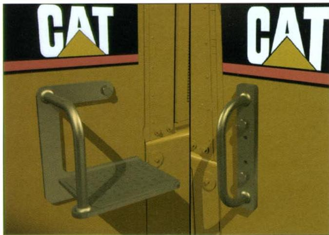
**Heavy duty steps and handles** are manufactured from plate steel and solid rod to withstand the rigors of landfill operation.
