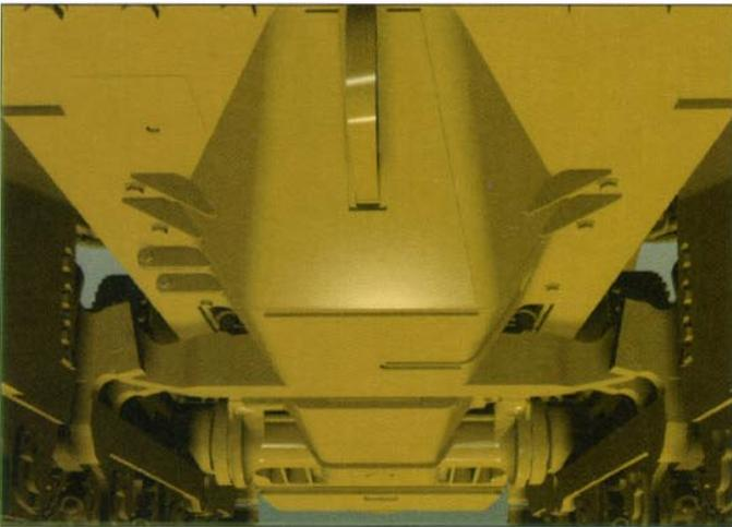
**Crankcase (belly) guards** serve a dual purpose. They help prevent contact damage to vital power train components, and help keep debris out of the power train compartments.
