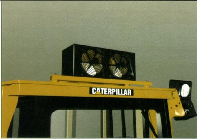
**ROPS-mounted air conditioner condenser and fans** are relocated from the engine compartment to the ROPS.
