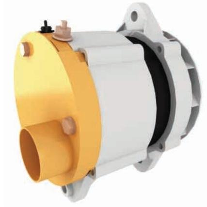
**High-capacity Ducted Alternator.** The high-capacity 95-amp alternator provides additional power required for electrical accessories such as supplemental lights and communications and entertainment radios. The ducting helps prevent debris from entering into the alternator.
