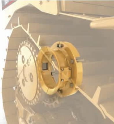
**Clamshell Guards.** The clamshell guard provides a non-rotating guard installed over the final drives to help prevent wire wrap. The guard includes inspection plates.
