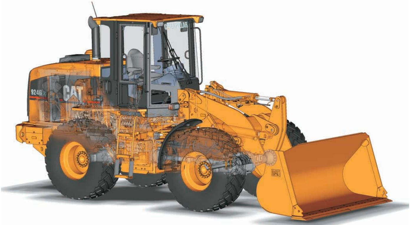
**Caterpillar Engine.** The six-cylinder 3056E Direct Injection Turbocharged (DIT) engine with Air-to-Air After Cooler (ATAAC) has a proven reputation for reliability, durability and performance. Fuel injection is electronically controlled for precise timing.
