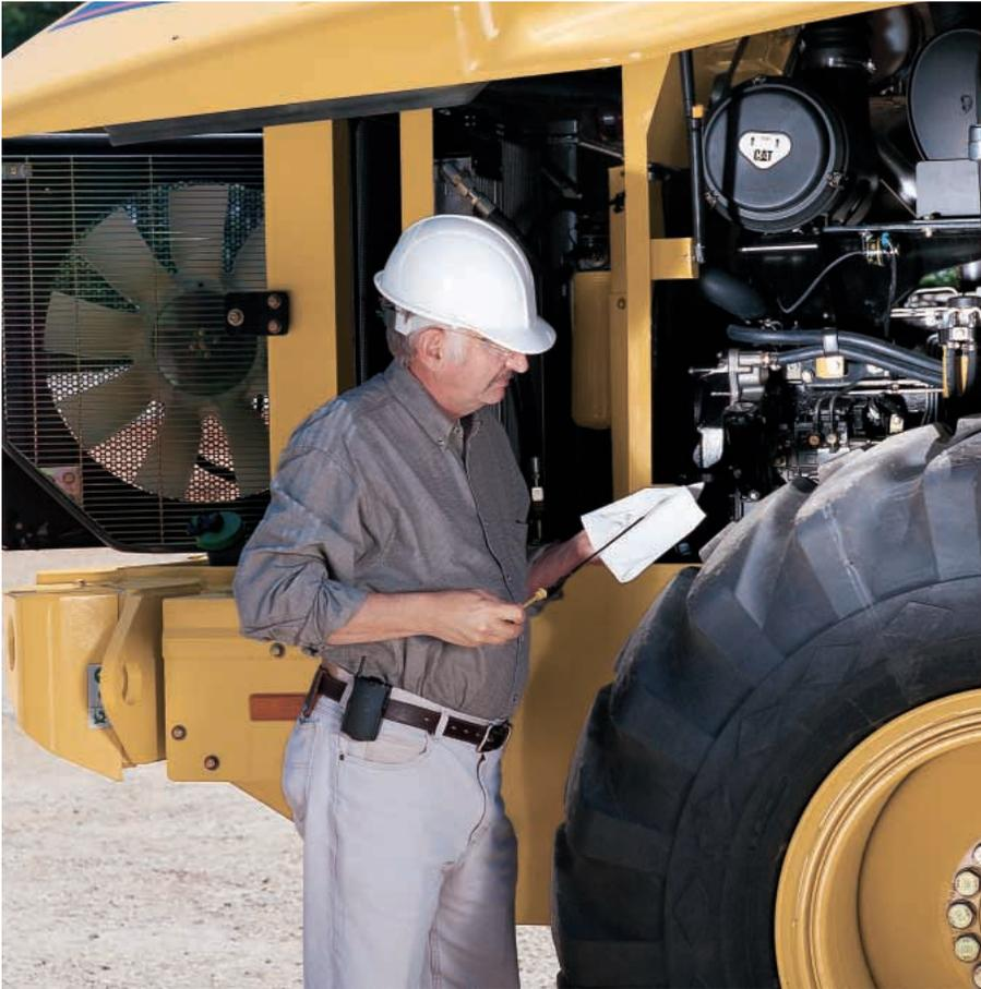
**Easy Access.** Gull-wing engine enclosure doors with gas struts lift for exceptional access to filters and service points. Radiator and oil coolers are easily accessible for cleaning.
