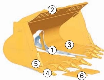
**Spade-Edge Rock Buckets with Bolt-On Segments.** Are available in 11.5 m<sup>3</sup> (15.0 yd<sup>3</sup>) and 12.3 m<sup>3</sup> (16.0 yd<sup>3</sup>) sizes. Each accepts up to two sets of sidebar protectors (5), features shouldered, double-strap adapters, easily changed bolt-on segments (6) and several tip options to provide good performance and serviceability.
