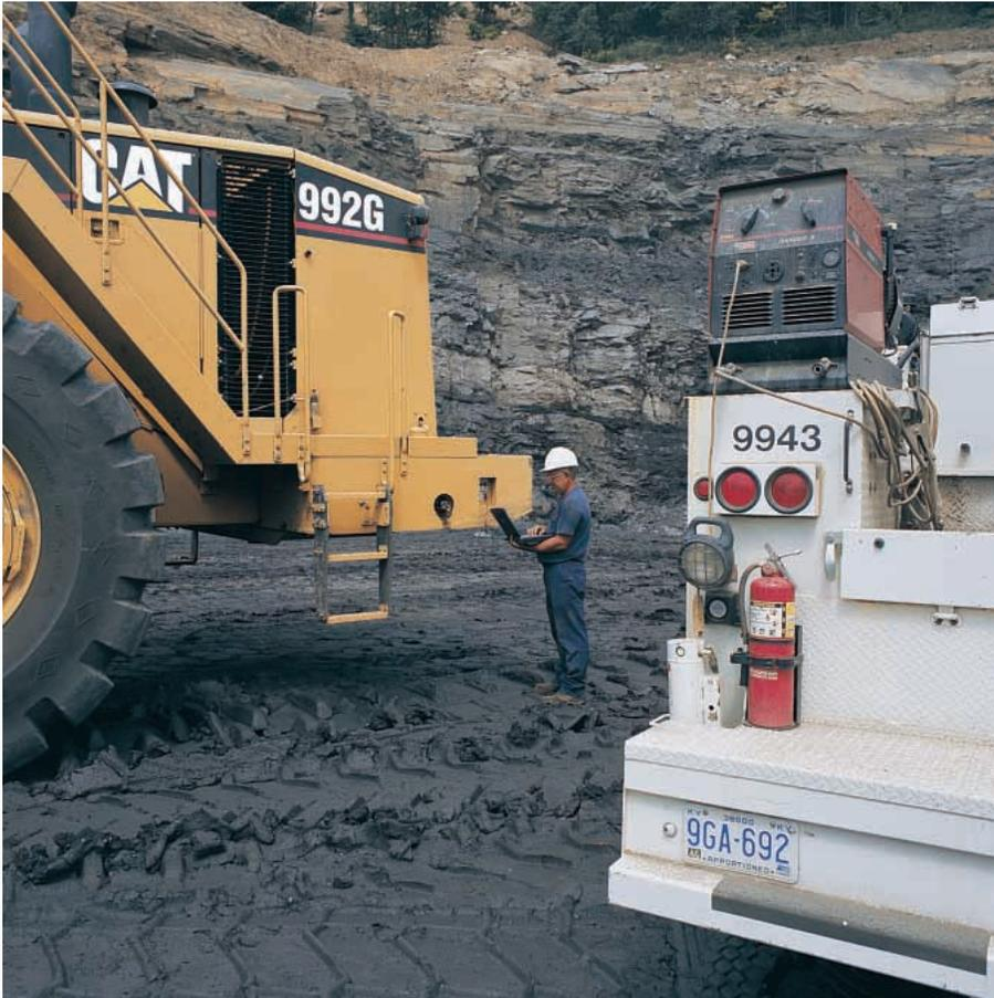
**Maintenance and Repair.** Is easier through monitoring key functions and logging critical indicators. Electronic diagnostic access is possible with a single tool, the Electronic Technician. In addition to the servicing features built into the engine, the 992G includes:
