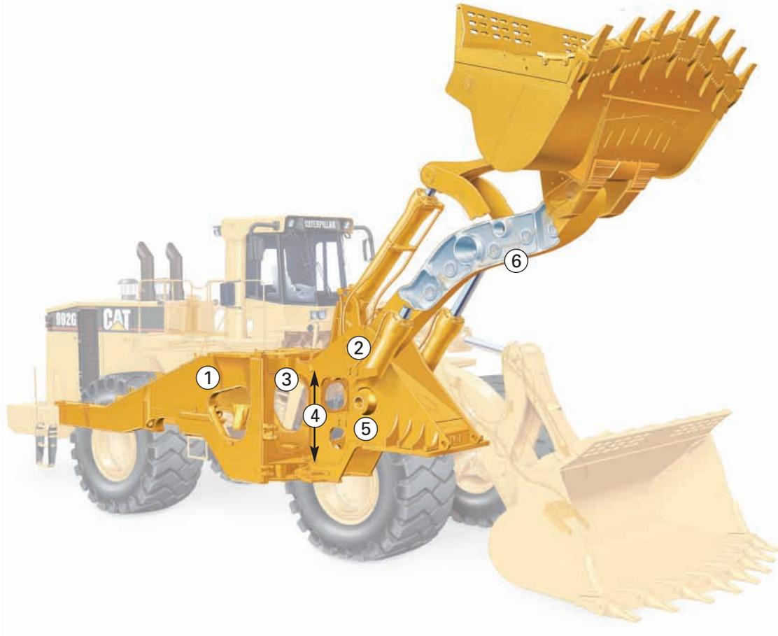
**Structures.** On the 992G, combine the use of robotic welding and castings in critical high-stress areas. More than 90 percent of the 992G structure is robotically welded to provide highly consistent welds and increased strength. Castings are also used in several areas to increase strength by helping to spread the loads and reduce the number of parts.
