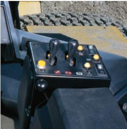
**Revolutionary Electro-Hydraulic Control System.** Uses separate hydraulic circuits for the lift/tilt/engine fan and steering/brake control. The benefits of the separate hydraulic systems are increased cooling and elimination of cross-contamination. XT-3™ and XT-5™ hose and reliable components help reduce the risk of leaks and blown lines, helping protect the environment.
