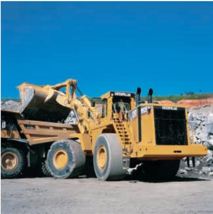
**Performance.** The 992G is an aggressive first gear loader for face and bank excavation. With increased dump clearance, the 992G can easily load off-highway, 90 metric tons (100 ton) trucks in four passes. The 992G HL is an excellent six-pass match for 136 metric tons (150 tons) off highway trucks. Increased performance and good pass match make the 992G a versatile performer with a cost per ton that will help your bottom line.
