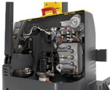
Sealed AC motor, controllers and connectors
