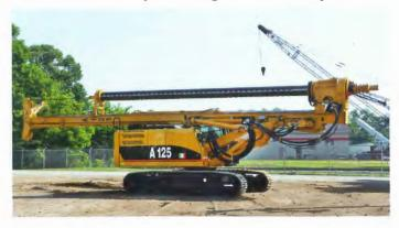
Kelly Tractor Co. recently introduced the new A125 drill rig to North America. Built in collaboration with IMT and Caterpillar OEM Solutions Group, the pioneering redesign enables the Tier 4 rig to lay flat for complete single load transport.
